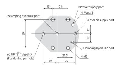
● The mounting surface finish must be no rougher than Rz6.3 (ISO4287:1997).
