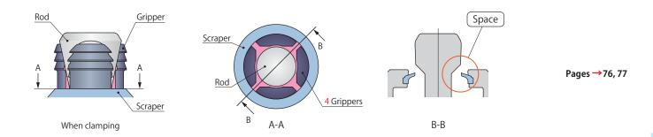
Because of space between scraper, gripper and the rod, air blow must always be performed to prevent intrusion of chips.
