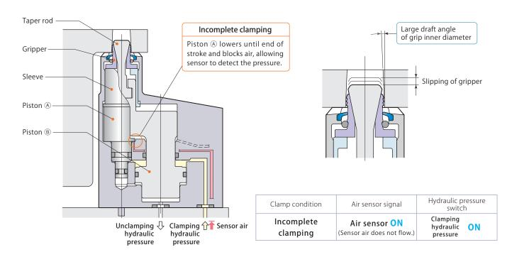
With the development of the non-constant air blow expansion clamp, air consumption will be significantly decreased. The traditional model ordinarily requires 50L/min (0.3MPa) flow rate (when grip inner diameter is ø12). The new model can reduce
