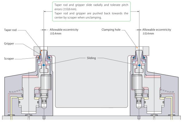
By the eccentric mechanism, the expansion clamp does not have a workpiece positioning function.
