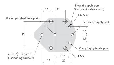
• The mounting surface finish must be no rougher than Rz6.3 (ISO4287:1997).
