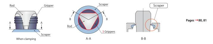
Because there is no space between scraper, gripper and the rod, it is not necessary to perform air blow during cutting process.
