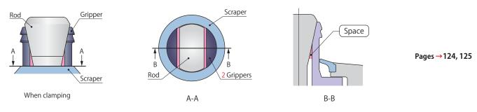
Because of space between scraper, gripper and the rod, air blow must always be performed to prevent intrusion of chips.
