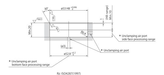
\*: Unclamping air port must be made on either side or bottom face.
