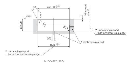
\*: Unclamping air port must be made on either side or bottom face.
