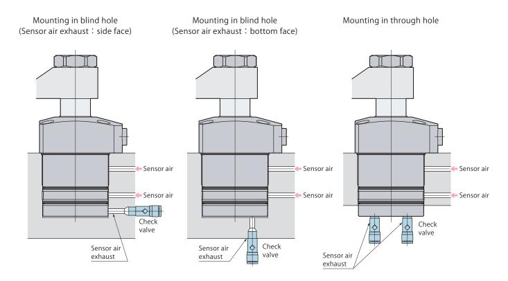
• Use a check valve with cracking pressure of 0.005 MPa or less if there is a risk of metal chips or coolant intrusion. Recommended check valve: AKH or AKB series manufactured by SMC.
