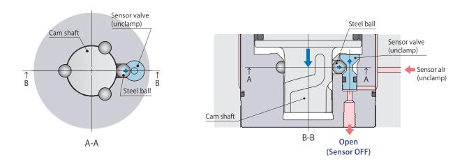
When the cam shaft lowers, the sensor valve (unclamp) is pushed up by the steel ball to open for air exhaust. CTM-B
