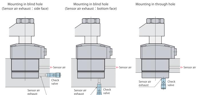
• Use a check valve with cracking pressure of 0.005 MPa or less if there is a risk of metal chips or coolant intrusion. Recommended check valve: AKH or AKB series manufactured by SMC.
