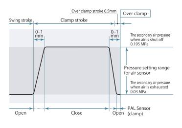
The diagram shown on the left indicates the relation between the PAL sensor, piston stroke, and secondary air pressure. (The pressure shown in the diagram is a reference based on the 0.2 MPa of primary air pressure for one piece of clamp.)
