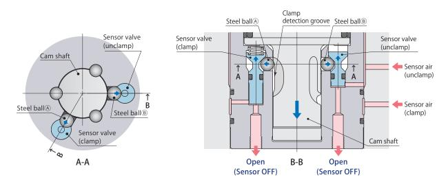
When the cam shaft passes the clamping point, the sensor valve (clamp) is pushed up by the steel ball
