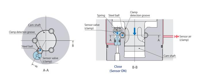
• The steel ball seats in the clamp detection groove when the cam shaft reaches clamping point, and a sensor valve (clamp) is pushed down to shut of the sensor air by a spring, and detects the clamped condition.
