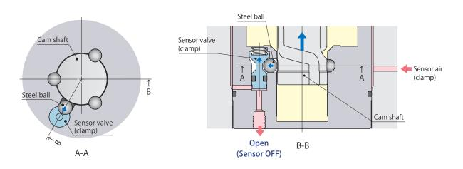
• The sensor valve (clamp) is pushed up by the steel ball to open for air exhaust while piston rod swing strokes.
