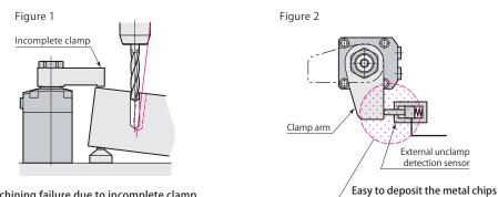
Machining failure due to incomplete clamp
