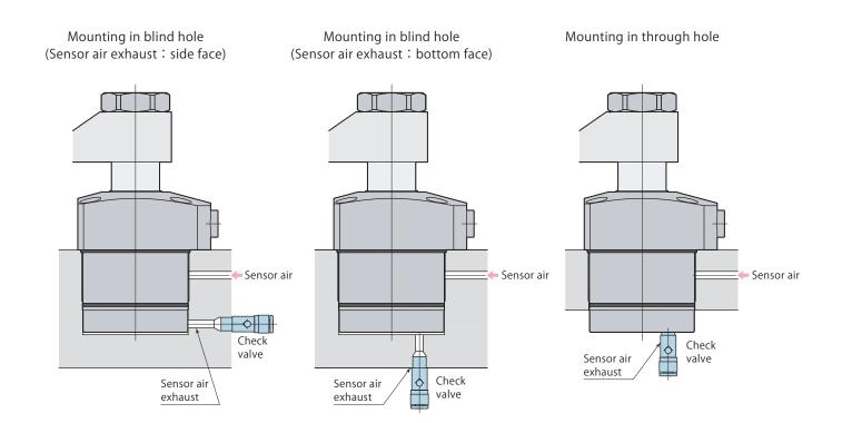
• Use a check valve with cracking pressure of 0.005 MPa or less if there is a risk of metal chips or coolant intrusion. Recommended check valve: AKH or AKB series manufactured by SMC.
