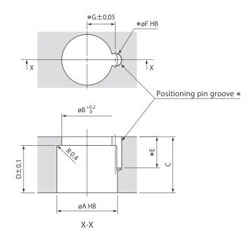
\*: No need to machine the pin groove (E, øF, G) unless positioning pin is used for the arm.The positioning pin enables a clamp arm to locate on the clamp firmly and easily.
